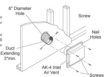
Figure 22 - Combustion Air Assembly for Model No. AK-4
